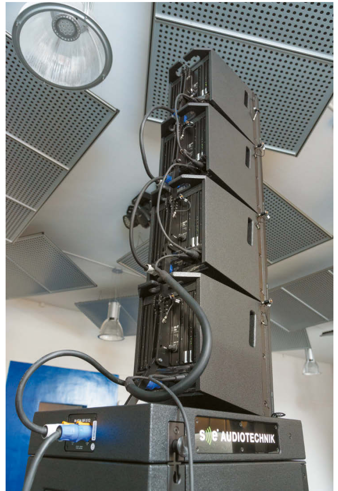
Through wiring of the tops we could have unfolded the rain cover a little bit better for the picture
